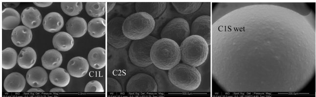
Figure 1. Scanning electron microscopy of C1L and C2S sorbent particles (dry state) and C1S (wet state, environmental scanning electron microscope).
